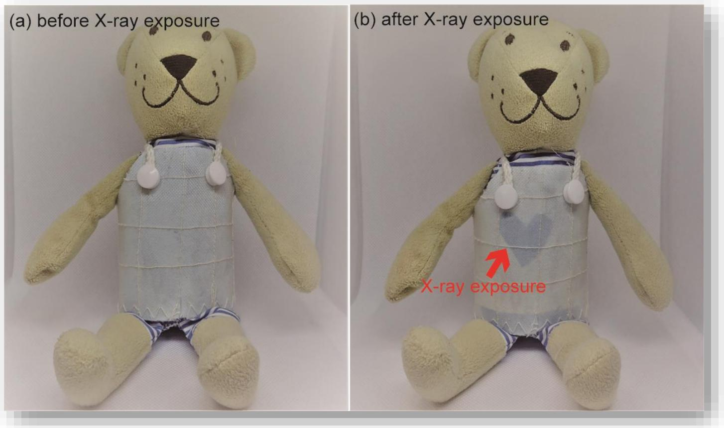
**Figure** Photographic images of the clothlike chromic dosimeter (a) before, and (b) X-ray exposure through the lead sheet cut in a “ $\heartsuit$ ” shape.
