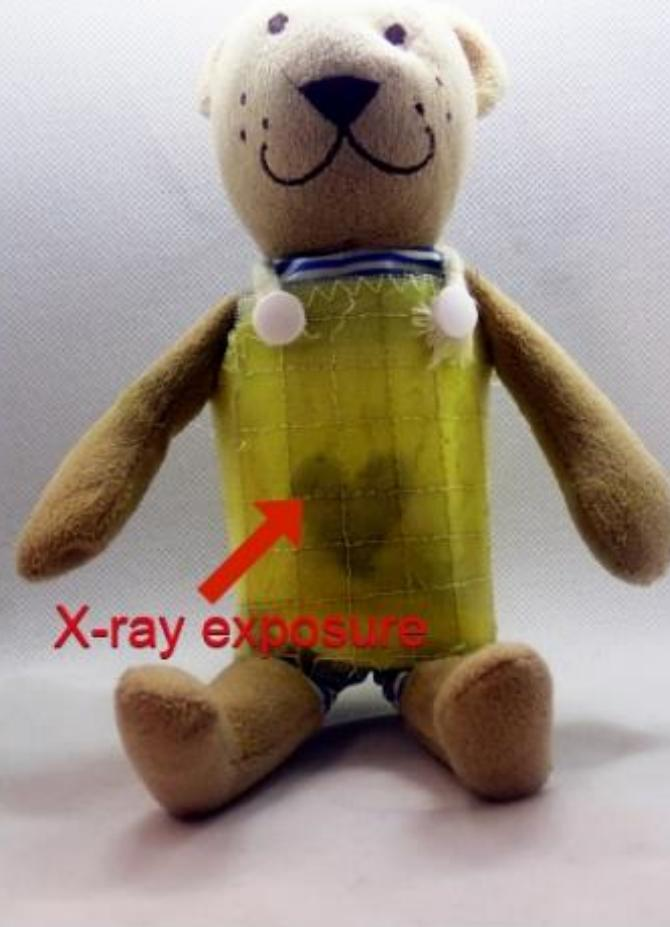
**Figure** Photograph showing aspect of the fibrous color dosimeter with MBTT/Black305 ratio at 3.0/3.0 w/w before and after X-ray exposure for 80 Gy. (e) Photographs of the clothlike fibrous color dosimeter with MBTT/Black305 ratio at 3.0/3.0 w/w (left) before and (right) after X-ray exposure through the lead sheet cut in a “♥” shape.
